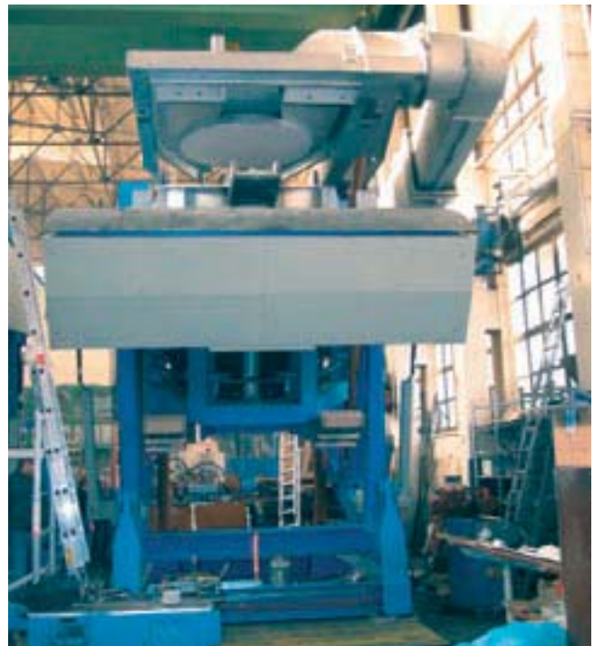
The 12-tonne furnace under shop assembly.
