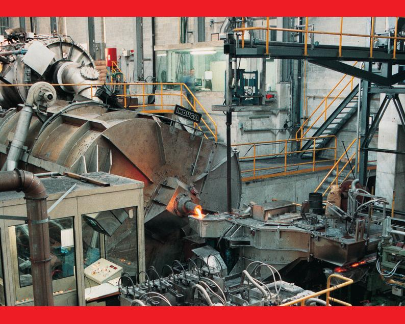
This induction heated alloying and metering furnace is an useful alternative solution to a conventional unheated tundish system. A very precise alloy adjustment, for example during the production of low-phosphorous DHP copper, combined with an good mixing and complete homogenisation of the melt are fundamental for casting high-quality copper grades
