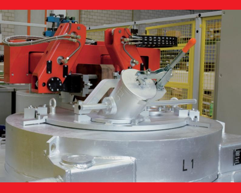
Automatic machine with 1 rotary manipulator and 1 furnace.
