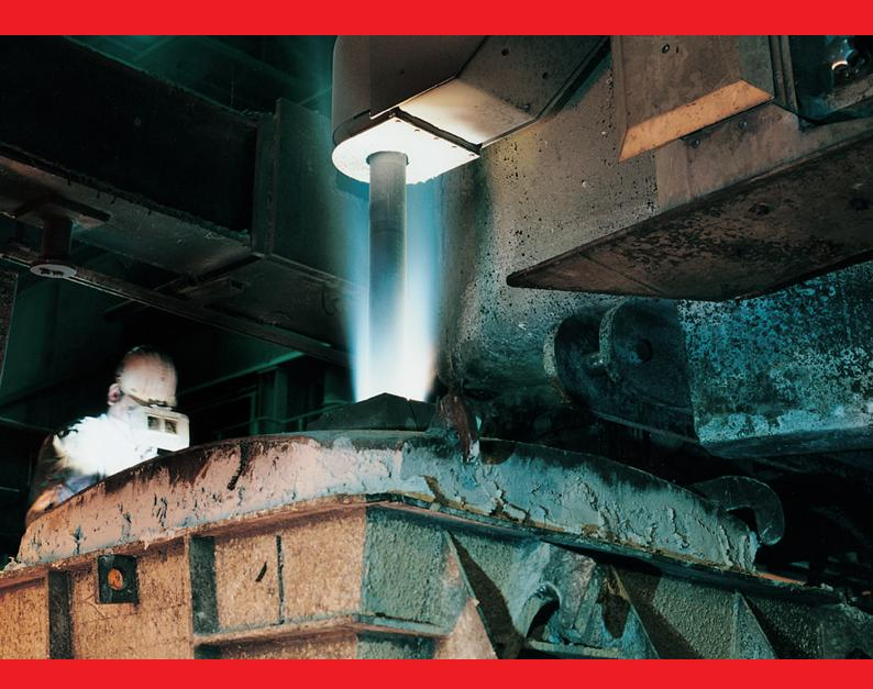
For the heating of liquid steel during continuous casting, INDUGA offers systems which heat the melt using electric plasma arcs. Depending on the application, the system can be operated with AC or DC power and special graphite electrodes. Excellent temperature control and a clean, carburisation-free heating are assured in all cases.
