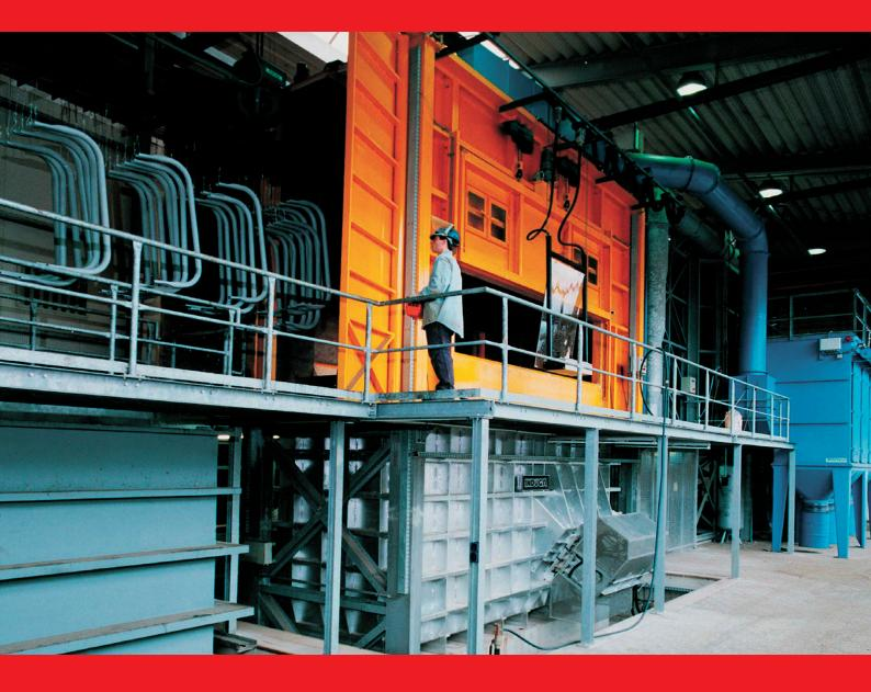
Galvanizing of pieces and large parts in an induction-heated ceramic lined furnace permits a flexible choice of high temperature coating in the range of about 620°C. The effects are optimum coating qualities in conjunction with very efficient operational results.
