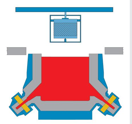
The induction heated channel-type furnace "coating pot", provides ideal preconditions for systematic temperature control within a broad range. Our expertise in arranging and dimensioning the channel inductors enables us to guarantee reliable operation with full compatibility and minimizing energy costs.
