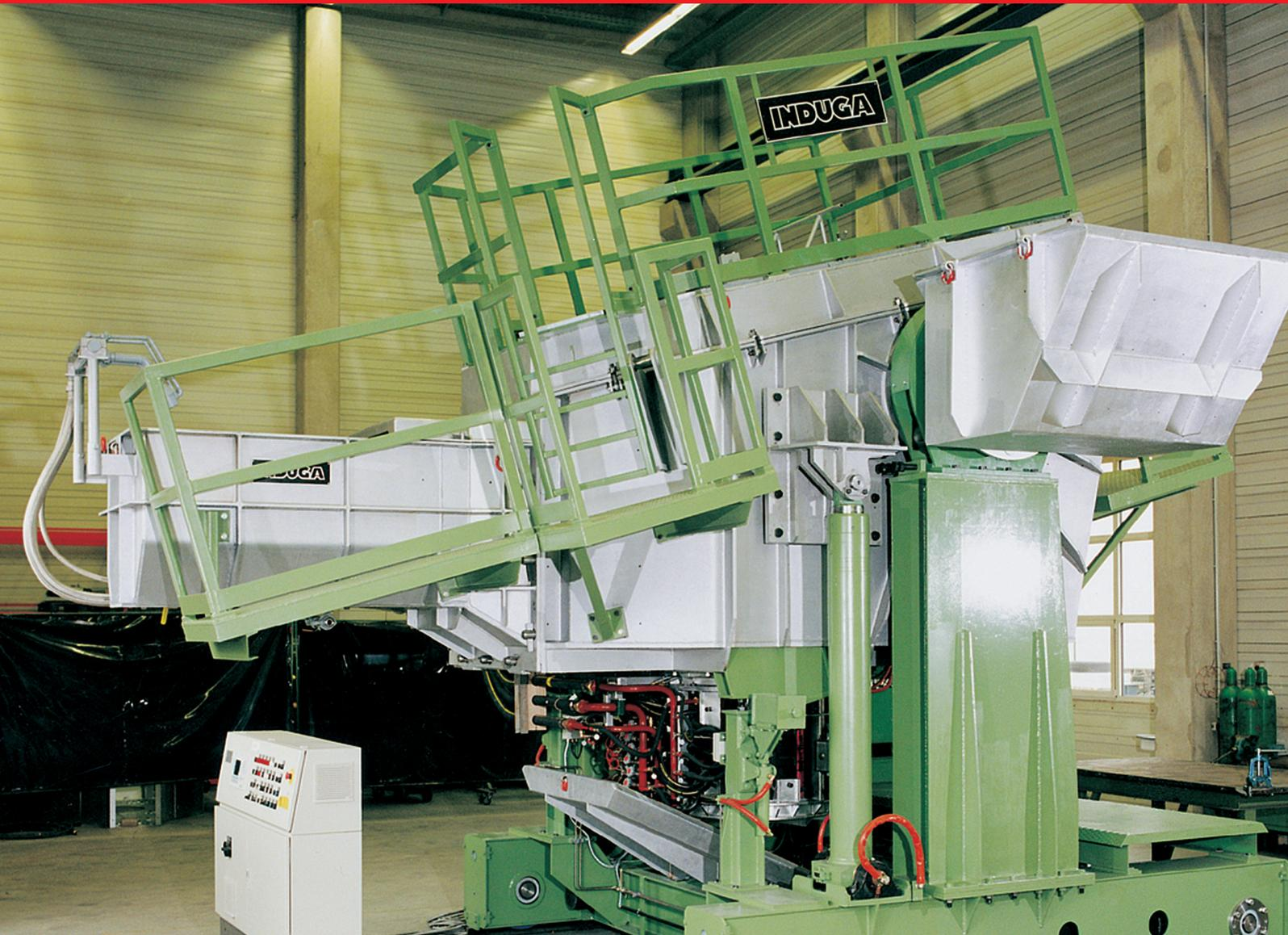
In order to be able to make use of the engineering benefits of the holding furnace with receiver for vertical casting also for customers that needs to change copper alloys very often, INDUGA offers this furnace type also with a crucible type inductor. This allows high flexibility for alloy changing and stable operation even with otherwise problematical alloys.
