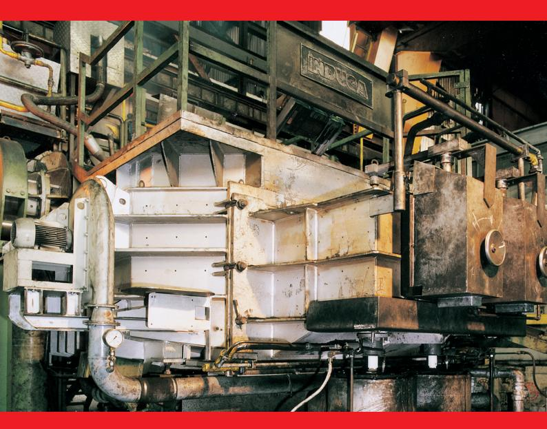
The demands made on the quality of the melt for the production of continuous cast semi-finished products are rising continuously. In order to guarantee the maximum utilisation of the casting lines, an adequate volume of liquid metal ready for casting with a constant temperature has to be supplied. To meet these demands, INDUGA has continuously optimised the induction heated holding furnace with receiver.
