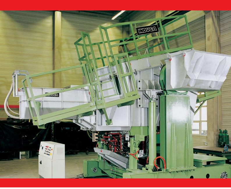
In order to be able to make use of the engineering benefits of the holding furnace with receiver for vertical casting also for customers that needs to change copper alloys very often, INDUGA offers this furnace type also with a crucible type inductor. This allows high flexibility for alloy changing and stable operation even with otherwise problematical alloys.
